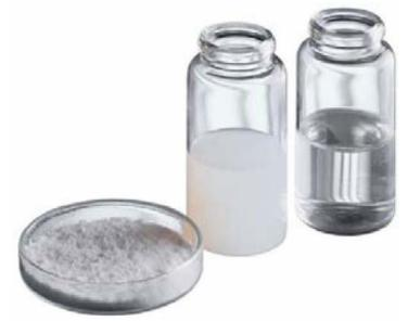
Liquid crystals exhibit characteristics between those of perfect crystalline order and the unstructured chaos of liquids. Macroscopically, the liquid crystalline phase behaves as a liquid. Microscopically, however, it resembles the solid phase since its physical characteristics are like those of a solid having anisotropic (i.e. directional) behavior. This is also reflected in the arrangements of the individual molecules.
