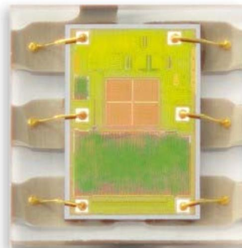
*TAOS makes a single-chip package that includes an ALS device and a proximity detector.*
